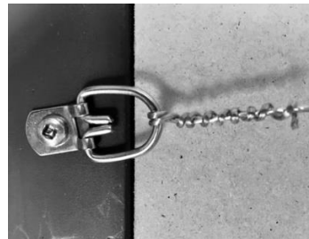
D-ring with coated wire twisted back around itself for about 1 inch. Before cutting your wires, leave enough room for the twist back. Uncoated wire must be taped on the ends to prevent injury.
